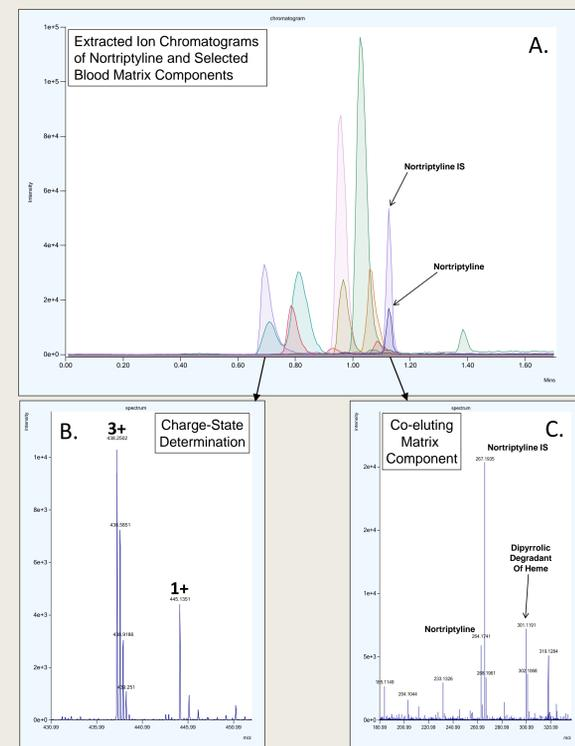
Figure 2. Selected extracted ion chromatograms (A) and mass spectra (B, C) of nortriptyline and matrix components eluting during LC-MS of a desorbed dried blood spot.
