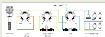
Figure 1. Schematic of the flow-through device and the PerkinElmer AxION 2 time-of-flight mass spectrometer.
