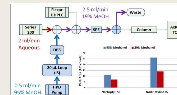
Figure 5. System schematic and, analyte and IS peak area with varied desorption solvent
