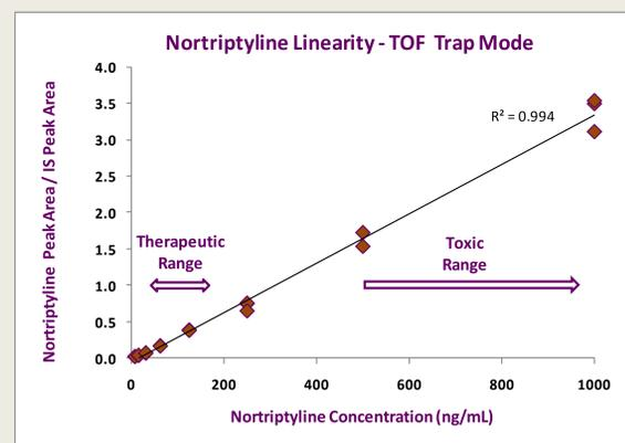
Figure 3. Nortriptyline linearity evaluated using the Spark Holland flow through device coupled online with the PerkinElmer AxION 2 LC-TOF MS
